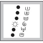
To select **Drain** press the **"Skip"** button three times, the **wash - rinse - spin** LED,s go out.
